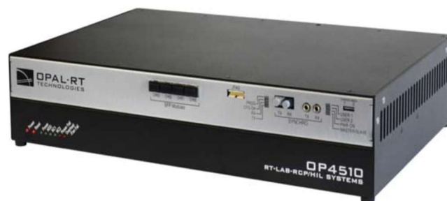
Figure 25. OPAL-Real Time Hardware-In-the-Loop (HIL) located in the authors' lab.
